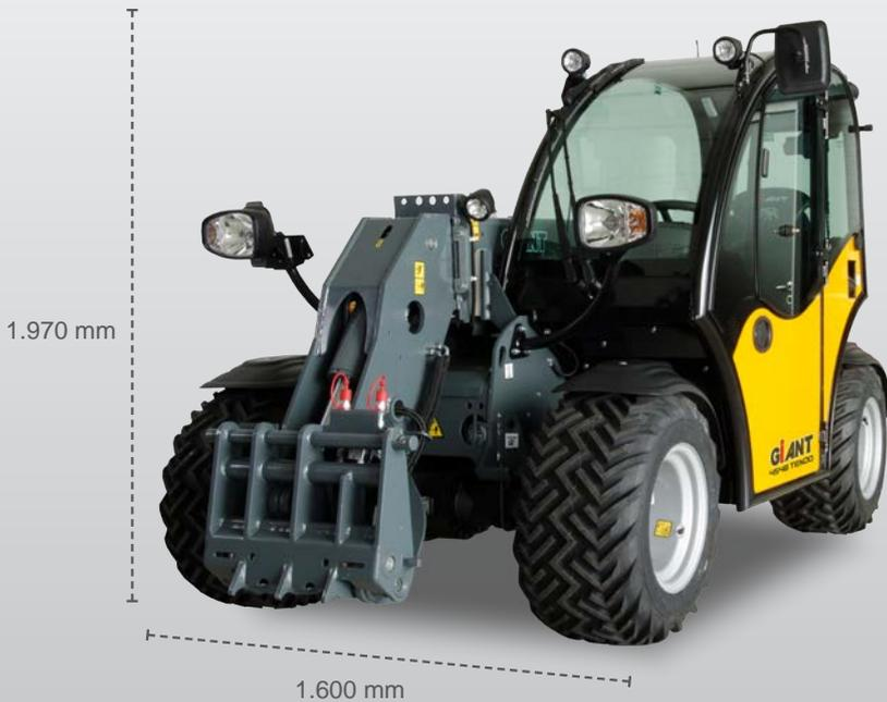
*The TENDO is extremely compact. It is narrower and less than two meters high. As a result, it manoeuvres easily in all kinds of areas.*
