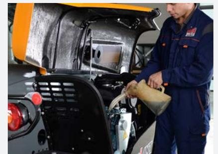
The engine compartment of the TENDO models are very accessible for daily checks of the oil, coolant and air filter.
