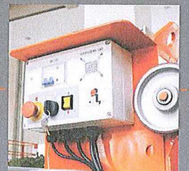
Ground control with outrigger LEDs
